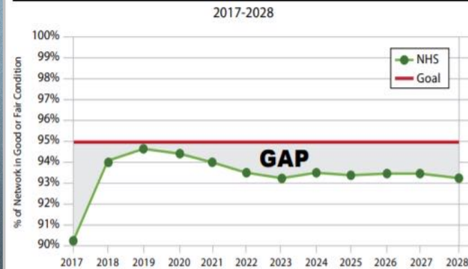
Figure 50: NHS Bridge Condition Gap
