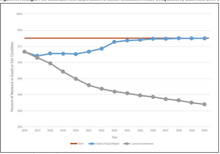
Figure 33: Michigan Non-Interstate NHS RSL/PASER Pavement Condition Forcast Comparison by Lane Miles 2016-2030
