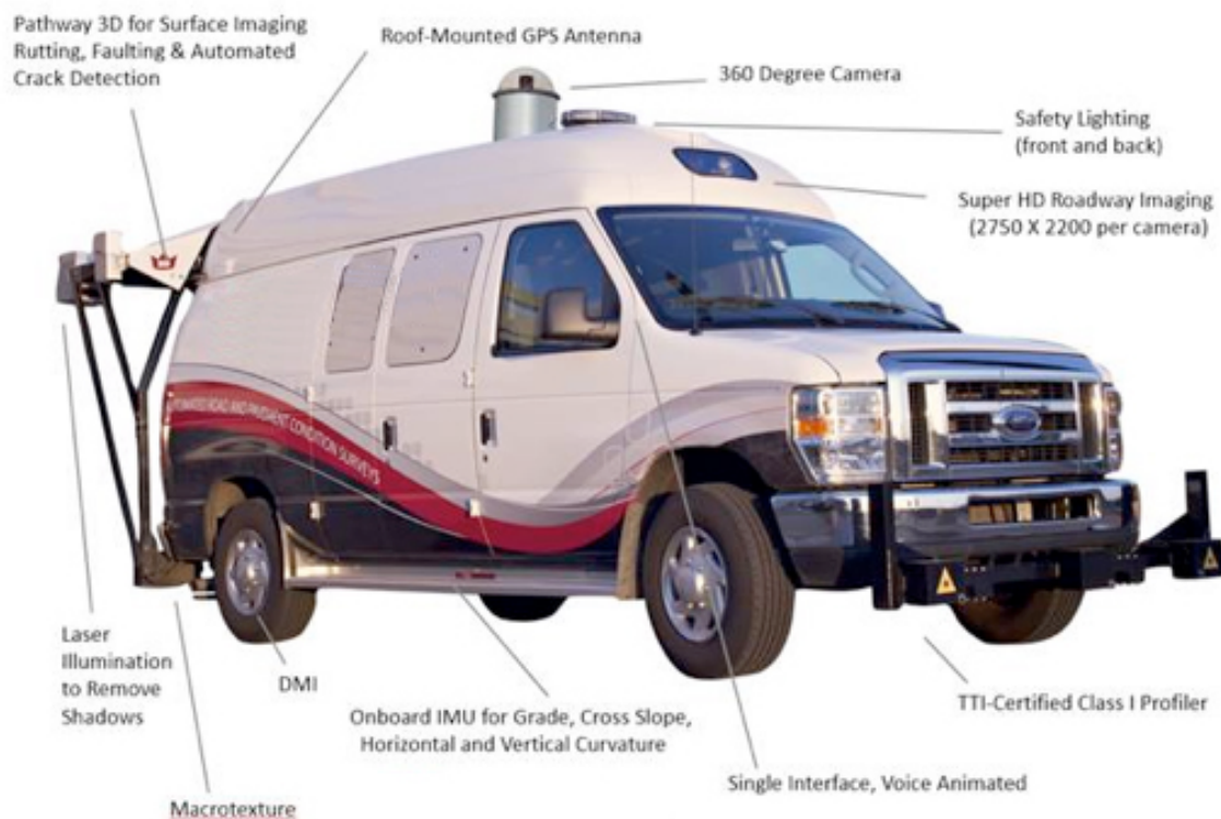
Figure 4-3. Automated Road and Pavement Condition Survey Van
