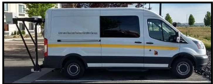
Figure 5-4: ITD's Profiler Van
