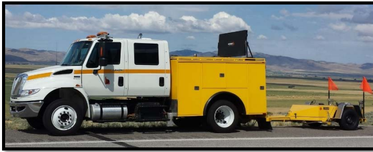
Figure 5-5: ITD's Pavement Friction Tester (PFT)
