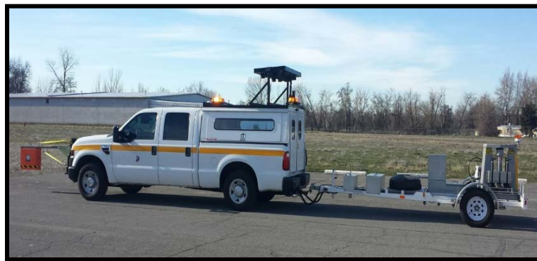
Figure 5-6: ITD's Falling Weight Deflectometer (FWD)
