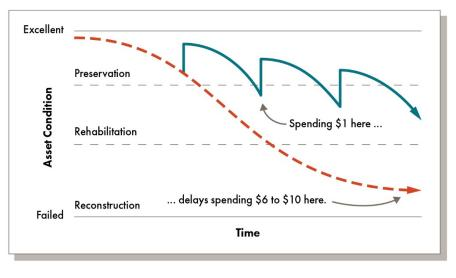
Figure 3-2. Example of pavement deterioration and treatment impacts.
