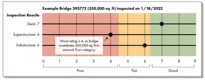
Figure 2-3. Example of a bridge performance rating.
