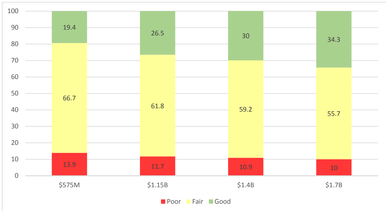
Figure 7.4 2027 NHS Bridge Conditions by Avg. Annual Funding
