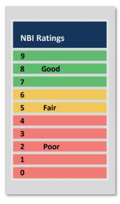
Figure 2-6. NBI Ratings for Bridge Condition
