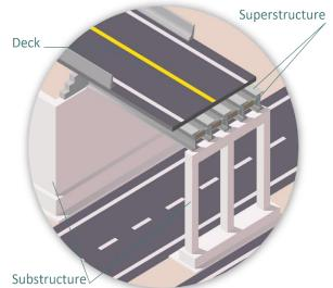
Figure 2-7. Bridge Components
