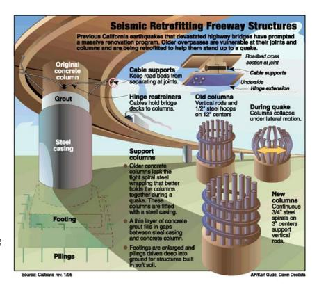
Figure 5-8. Seismic Retrofitting Freeway Structures Infographic
