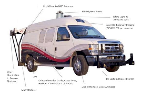
Figure 4-3. Automated Road and Pavement Condition Survey Van
