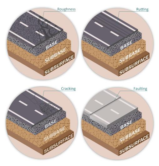
Figure 2-5. Pavement Condition: Four Metrics
