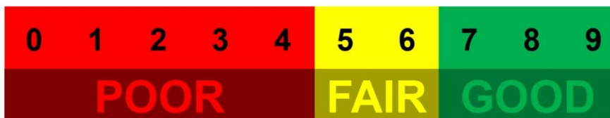
Figure 8: National Bridge Inspection Rating Scale
