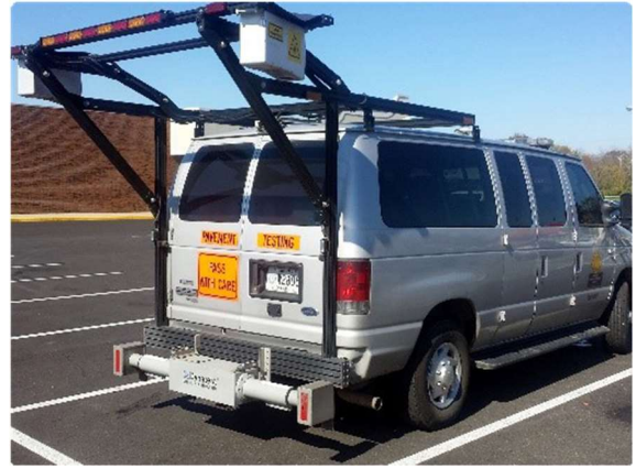
Figure 3-13. KYTC's automated pavement data collection equipment
