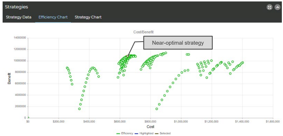
Figure 4-5: PMS cost benefit analysis results for multiple investment strategies for one pavement segment
