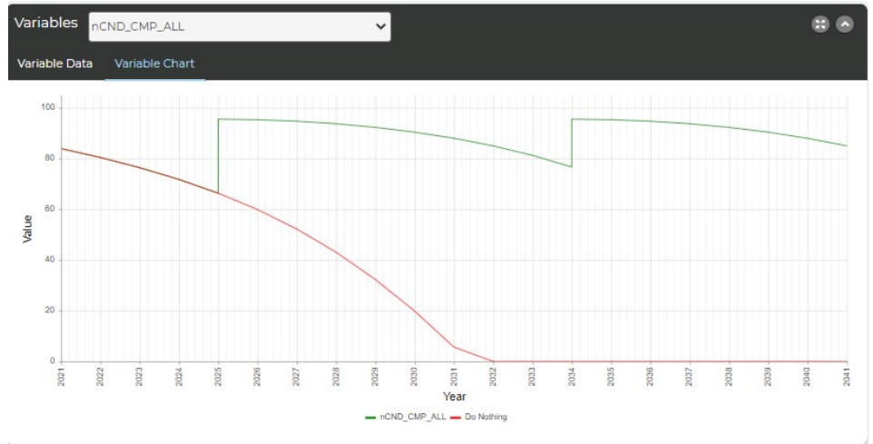
Figure 4-3: An example of one of many treatment strategies for a pavement in Good to Fair condition generated by PMS
